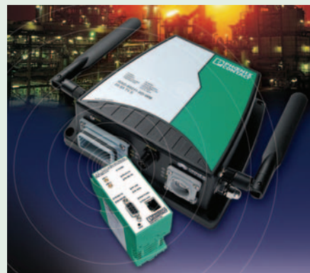
Wireless Ethernet radio, like this from Phoenix Contact, is replacing hard-wired networks in industrial facilities.
